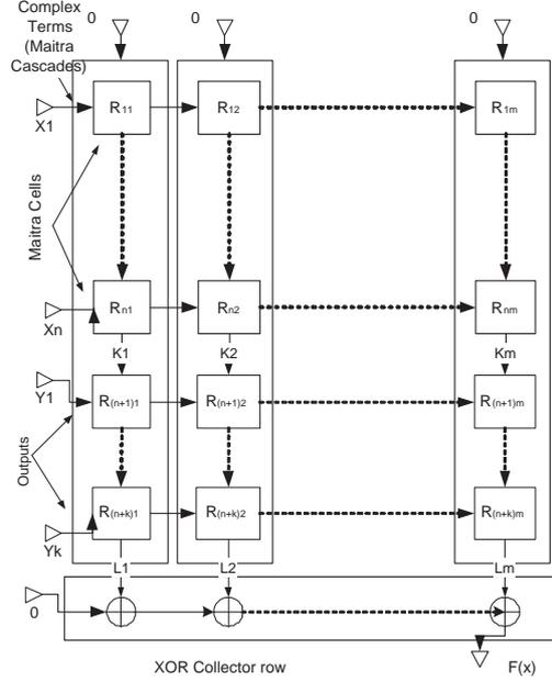
Figure 2: 1st algorithm multi-output architecture
