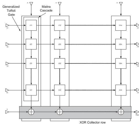
Figure 1: Reversible wave cascade architecture
