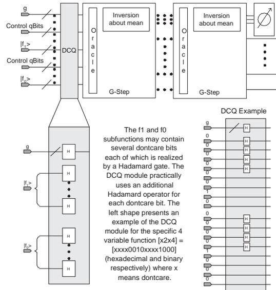
Fig. 5. DCQmin-Oracle Circuit with example
